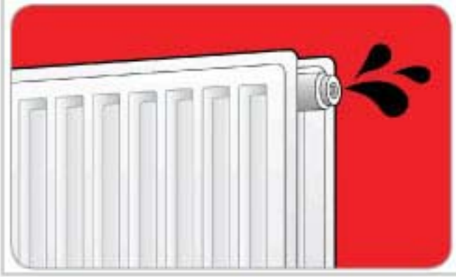
Dirty black or brown water present when bleeding radiators confirms system corrosion.
